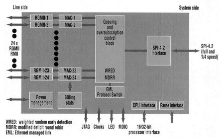
The A2510 Harrier chip offers 24 ports capable of 10/100/1000-Mbit/s traffic on one side and a 10-Gbit/s SPI-4.2 interface on the other. Its intelligent buffering scheme combines the 24 ports of traffic (up to 24 Gbits/s) into one 10-Gbit/s stream or unpacks a 10-Gbit/s stream into 24 separate 1-Gbit/s streams.
